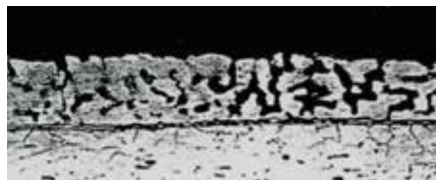
Microscopic picture view of ZINCALUME® steel after weathering
